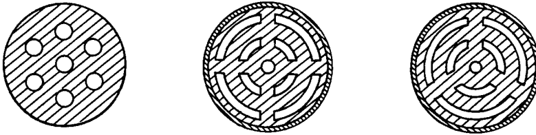
Figure 25.—Typical multiperforated grain shapes.
