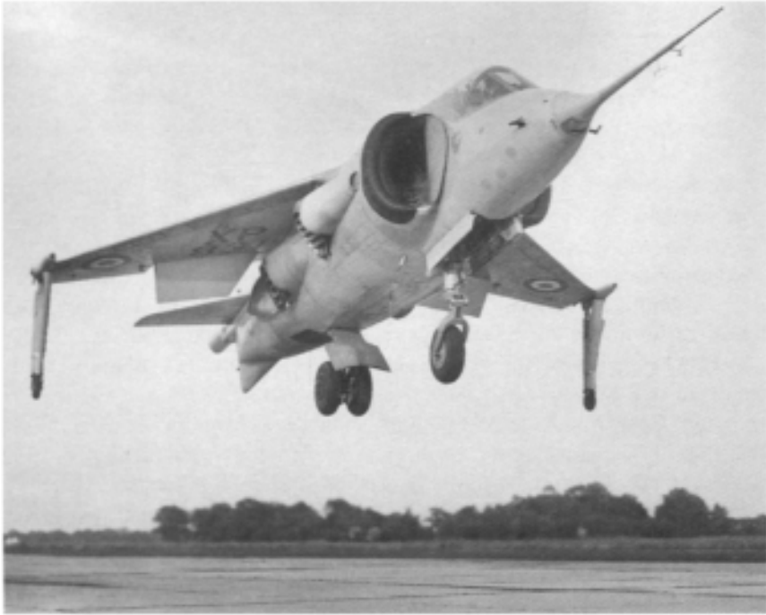
Figure 12.12: The Hawker P.1127 supported by the thrust from the four deflected jets produced by its Bristol Pegasus engine. Hawker Aircraft photograph.
