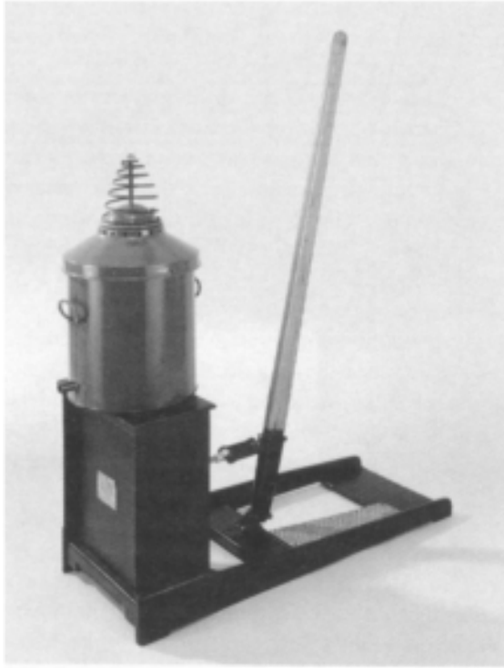
Figure 19.4: Sir Hiram Maxim's 'Little Giant' dust extractor, 1909. Dust is trapped in the canister which contains sawdust as a filter. Suction obtained by working long handle. Canister stands on top of a diaphragm pump. The springloaded valve in the lid acts as a safety valve and measure of suction is obtained. Price in 1909 5 guineas.
