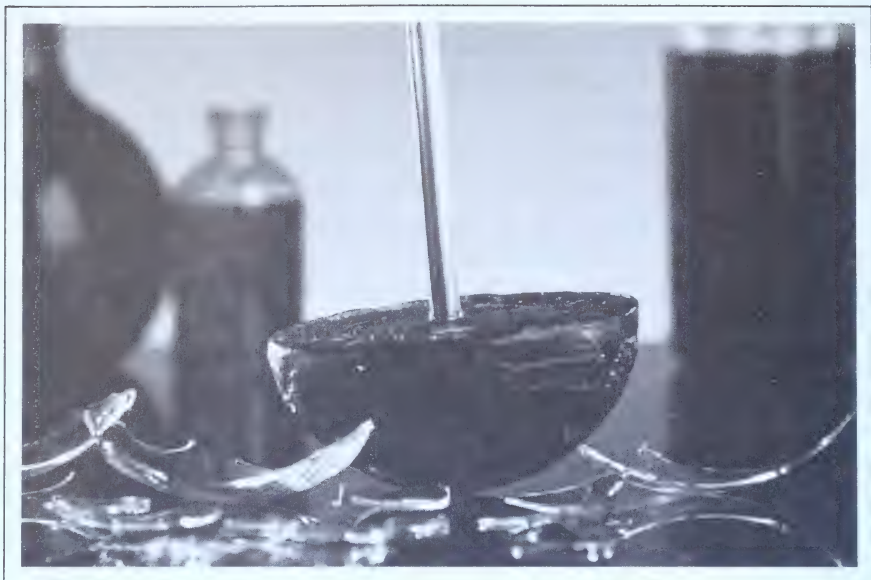
▼ The first polycarbonate resin, formed around a stirrer in a glass flask that had to be broken away from it
