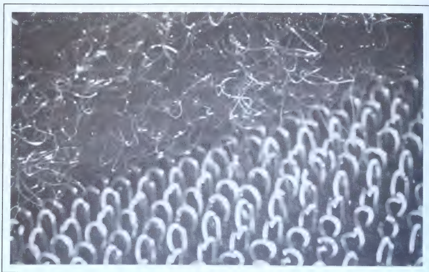
▼ A photomicrograph showing the hooks and loops, the fundamental components of Velcro Brand fasteners
