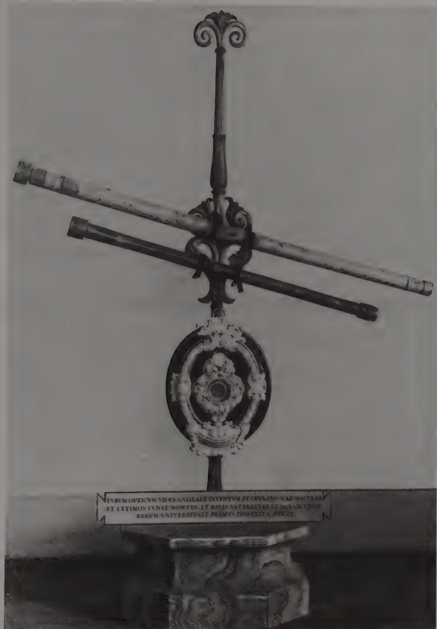
One of Galileo's telescopes. Galileo did not invent the telescope, but he did build his own based on what he had heard about how they worked. (AIP Emilio Segrè Visual Archives, E. Scott Barr Collection)
