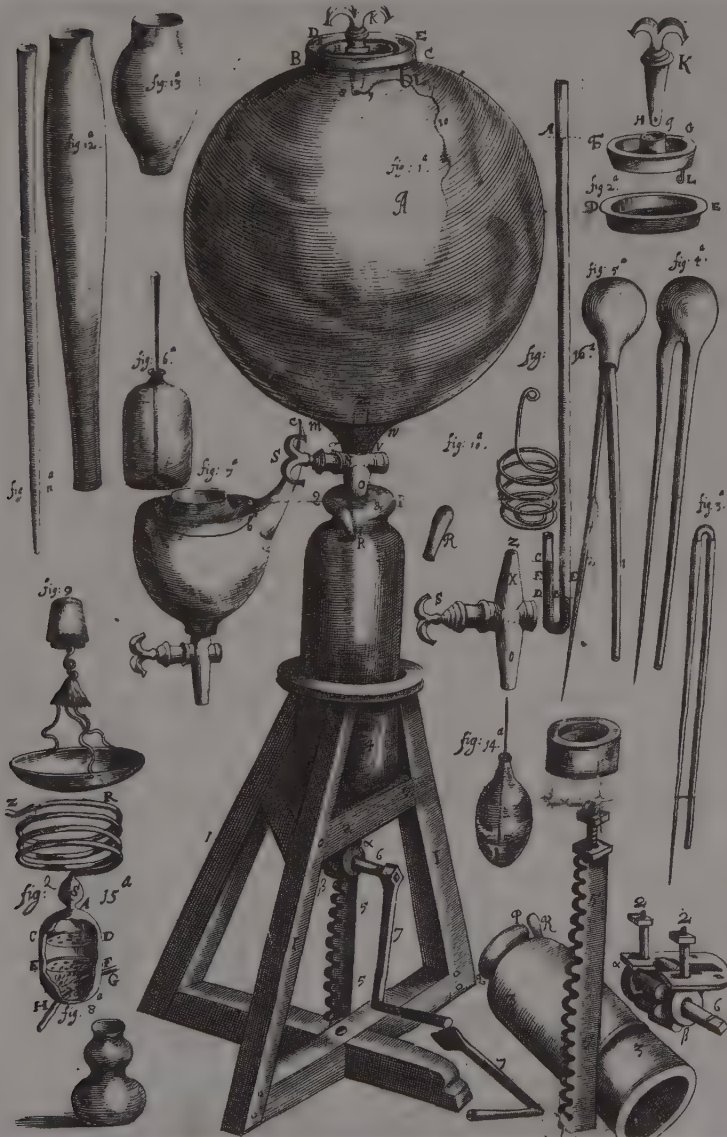
Air pump built by Robert Hooke for Boyle's experiments with a vacuum (Bancroft Library, University of California, Berkeley)
