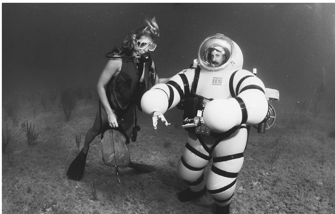
THIS YELLOW DIVING SUIT, CALLED A “NEWT SUIT,” IS SPECIALLY DESIGNED TO WITHSTAND THE ENORMOUS WATER PRESSURE THAT EXISTS AT LOWER DEPTHS OF THE OCEAN. (Photograph by Amos Nachoum/Corbis. Reproduced by permission.)
