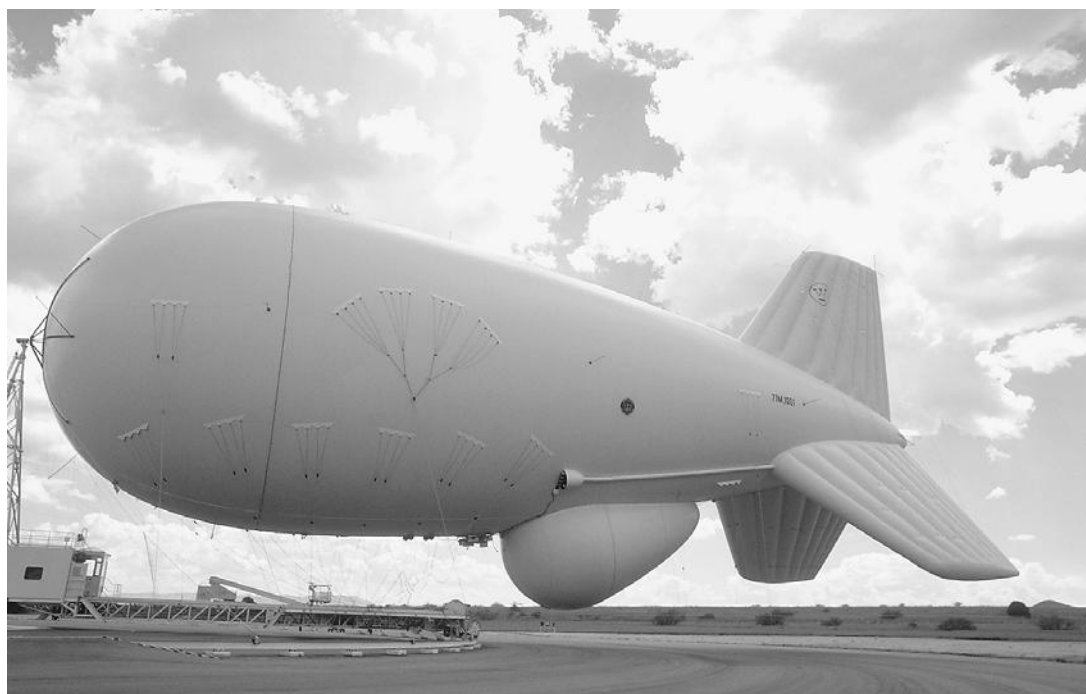
ONCE CONSIDERED OBSOLETE, BLIMPS ARE ENJOYING A RENAISSANCE AMONG SCIENTISTS AND GOVERNMENT AGENCIES. THE BLIMP PICTURED HERE, THE AEROSTAT BLIMP, IS EQUIPPED WITH RADAR FOR DRUG ENFORCEMENT AND INSTRUMENTS FOR WEATHER OBSERVATION. (Corbis. Reproduced by permission.)
