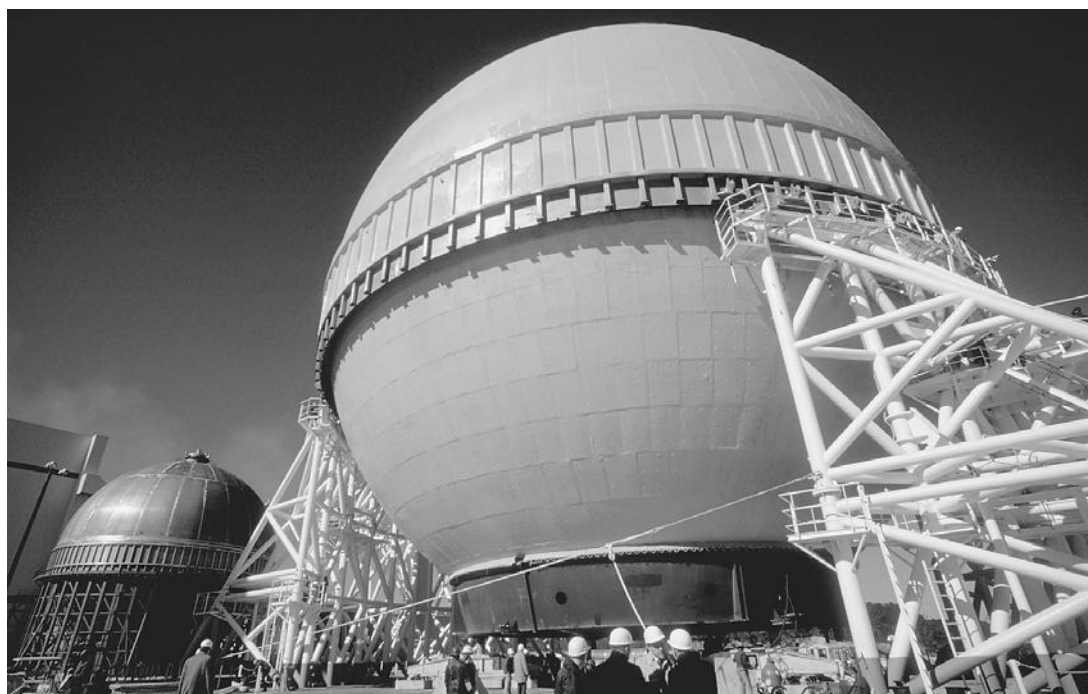
THIS HUGE LIQUEFIED NATURAL GAS CONTAINER WILL BE INSTALLED ON A SHIP. THE VOLUME OF THE LIQUEFIED GAS IS FAR LESS THAN IT WOULD BE IF THE GAS WERE IN A VAPORIZED STATE, THUS ENABLING EASE AND ECONOMY IN TRANSPORT. (Photograph by James L. Amos/Corbis. Reproduced by permission.)
