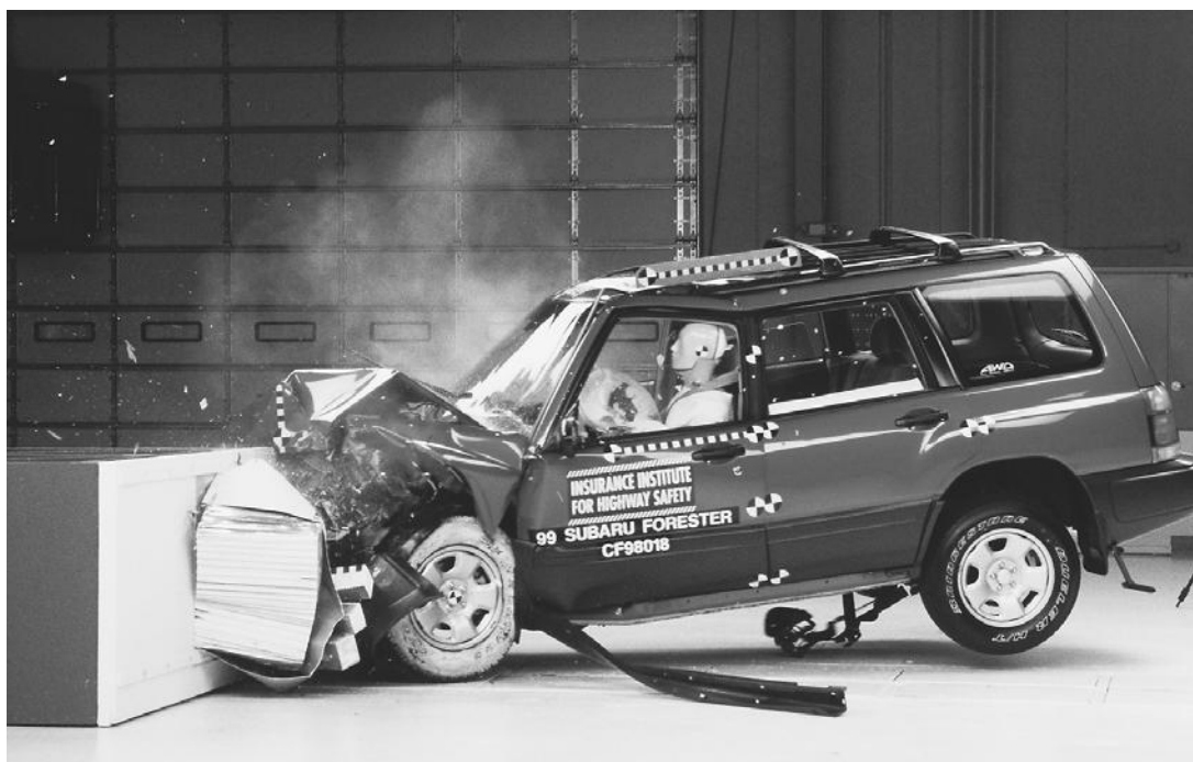
WHEN A VEHICLE HITS A WALL, AS SHOWN HERE IN A CRASH TEST, ITS MOTION WILL BE STOPPED, AND QUITE ABRUPTLY. BUT THOUGH ITS MOTION HAS STOPPED, IN THE SPLIT SECONDS AFTER THE CRASH IT IS STILL RESPONDING TO INERTIA: RATHER THAN BOUNCING OFF THE BRICK WALL, IT WILL CONTINUE PLOWING INTO IT. (Photograph by Tim Wright/Corbis. Reproduced by permission.)
