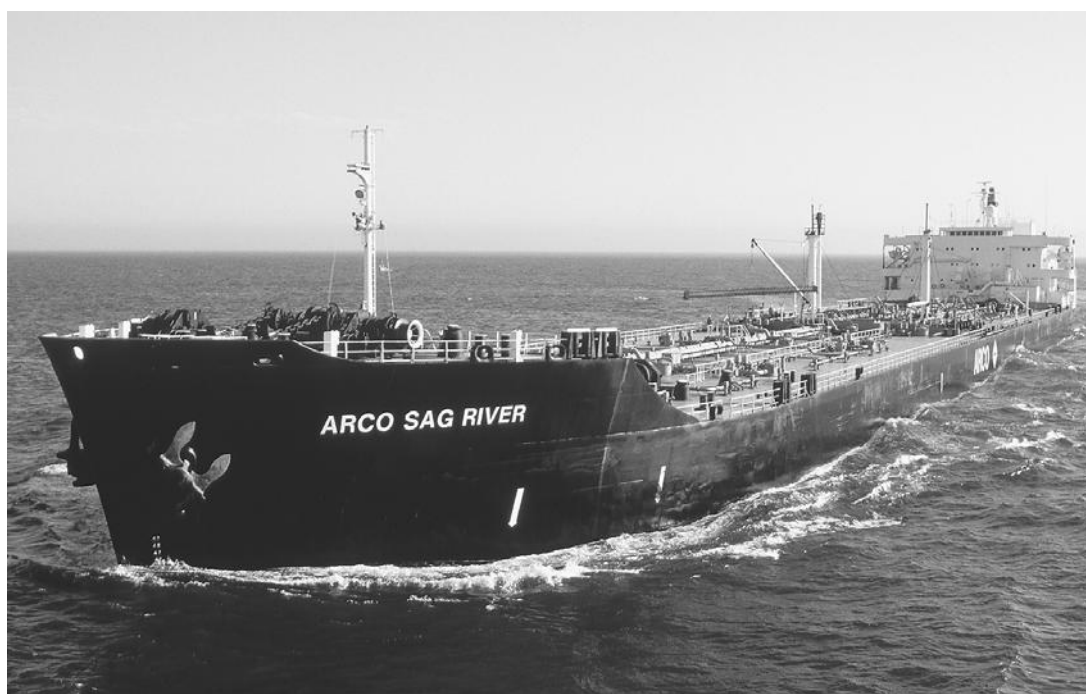
HOW DOES A GIGANTIC STEEL SHIP, SUCH AS THE SUPERTANKER PICTURED HERE, STAY AFLOAT, EVEN THOUGH IT HAS A WEIGHT DENSITY FAR GREATER THAN THE WATER BELOW IT? THE ANSWER LIES IN ITS CURVED HULL, WHICH CONTAINS A LARGE AMOUNT OF OPEN SPACE AND ALLOWS THE SHIP TO SPREAD ITS AVERAGE DENSITY TO A LOWER LEVEL THAN THE WATER. (Photograph by Vince Streano/Corbis. Reproduced by permission.)
