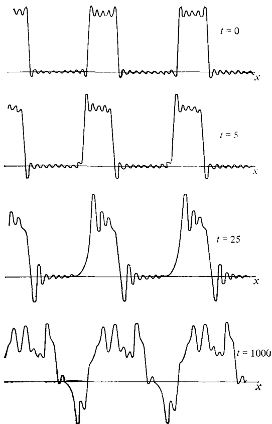
Fig. 21. A change in the shape of a wave in the course of time in a medium with strong dispersion. The numbers attached to the graphs correspond to conditional time 'instances' t .
