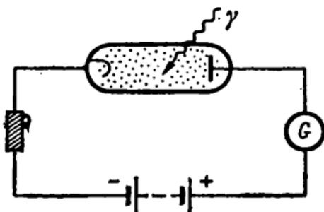
Fig. 50. A Geiger counter block diagram is placed in a protective housing with a window to enable it to work in a particular direction.
