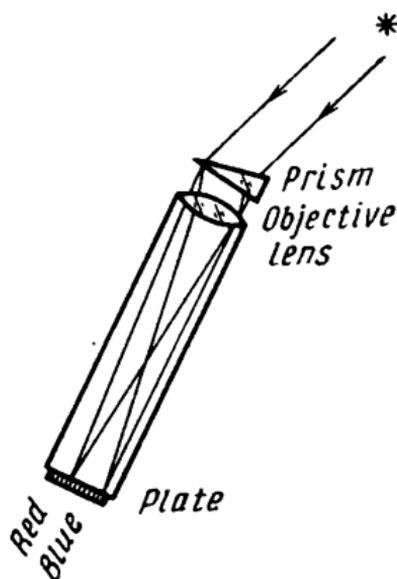
Fig. 80. A spectrograph with an objective prism
