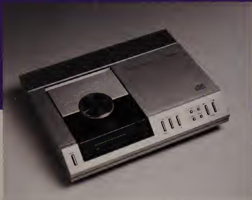
A CD player from 1983 made by Philips of Holland. The CD was developed by Philips in conjunction with the Japanese manufacturer Sony, and was first released in 1982. The rise of the CD reissues in the late 1980s and early 1990s was a boon to the record industry. At the time, these units were cutting-edge technology, lauded for their compact size and audio fidelity.
