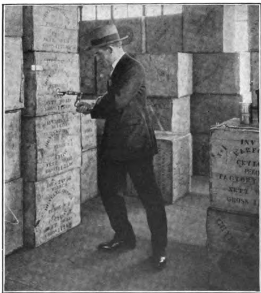
Boring sample hole with special auger.
