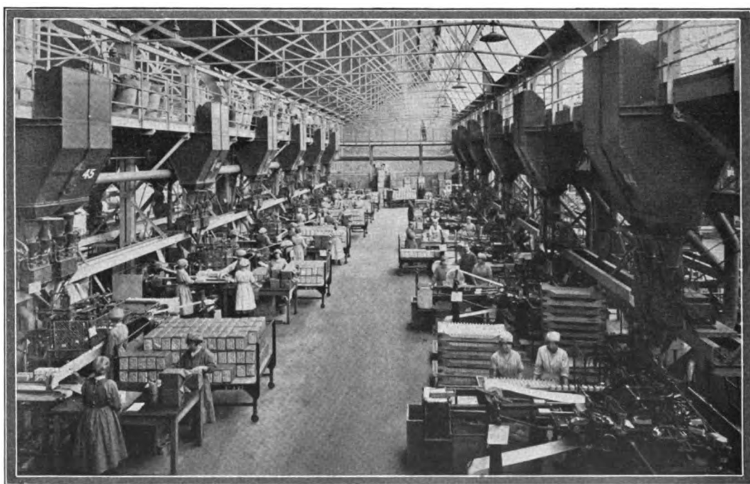
PACKETING ROOM, SHOWING TWELVE AUTOMATIC UNITS FED FROM MEZZANINE HOPPERS
