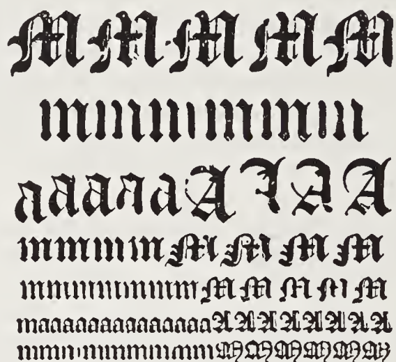
FIG. 2. Variations in the face of type produced by bad casting.
