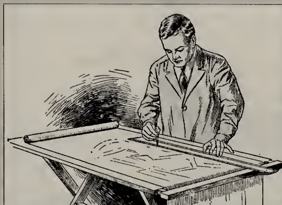
7-14. Designers used to work with t-squares, triangles and rubber cement to layout "galleys" received from phototypesetters. Once everything was measured, glued down, and instructions were written for the printer, the boards were shot as negatives and then burned into plates which were hung on the press and printed.
