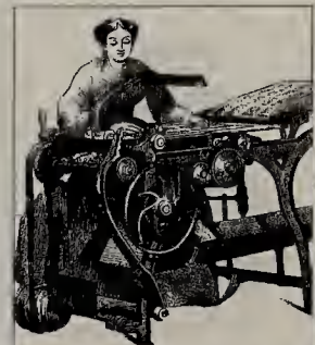
4-55. This historic drawing shows a woman operating a platen style, sheet-fed letterpress.
