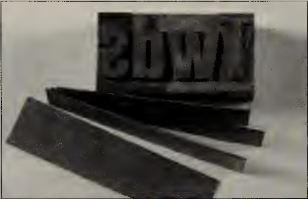
8-14. This photo of actual lead type above shows a few strips of leads standing up, and one lying down. The leads were placed between lines of copy to space out the lines, hence the word “leading” for line spacing.
