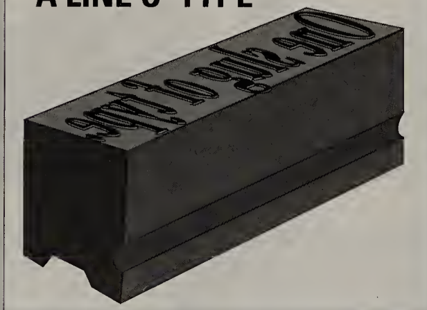
7-13. Above is a diagram of a line of type, cast as one piece from a linotype machine.
