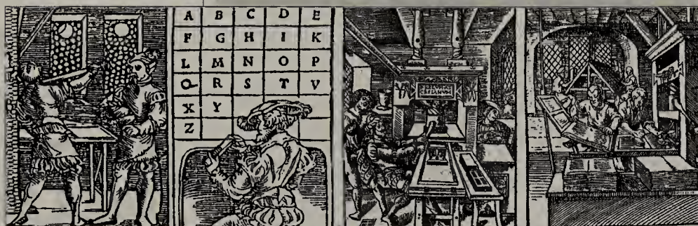
3-22. Printing shops sprang up across Europe in a flurry. There were almost two hundred print shops across Europe during the early 1500s. The woodcuts above show compositors on the left, the press being operated in the middle, and the inking of type on the right.
