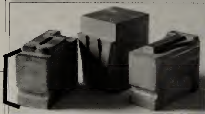
8-10. These actual pieces of lead type show the consistency of type high, and how the width of individual characters varied. You can also see that the ascender and descender areas had to be included in the piece of lead type, whether the letter had them or not, so that all of the type would line up evenly.
