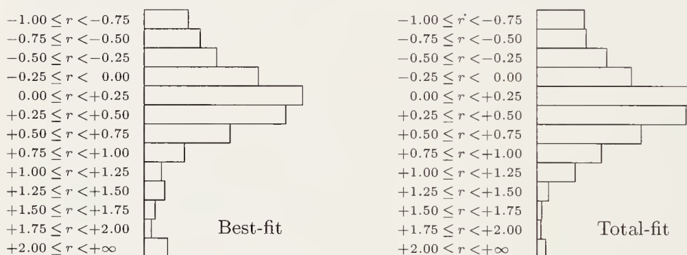
FIGURE 20. The distribution of interword spaces found by the best line-at-a-time method, compared to the distribution found by the best paragraph-at-a-time method, when difficult mathematical copy is typeset without human intervention.
