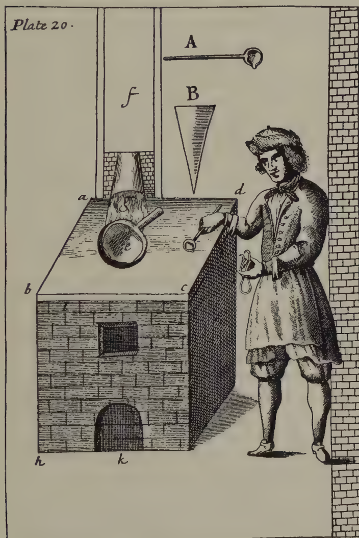
Typecasting by hand. From Moxon's "Mechanick Exercises" (1683-6), an early manual on printing and typefoundry
