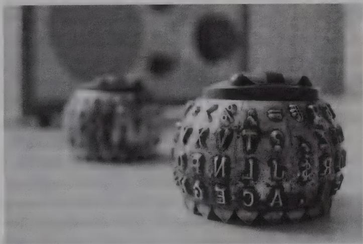
The IBM Selectric’s secret weapon – its inner golfball (about the size of a £2 coin)
