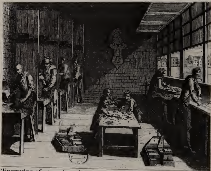
'Engraving of a type foundry presumed to be Caslon's, showing four letter casters at work, four boys breaking off types from surplus metal, a rubber and a dresser. Two halves of enlarged type mould are on the floor'. From The Universal Magazine , Vol.vi, 1750. (photo: St. Bride Printing Library)
