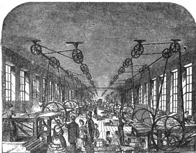
Pressroom of 1865, showing Adams presses in use
