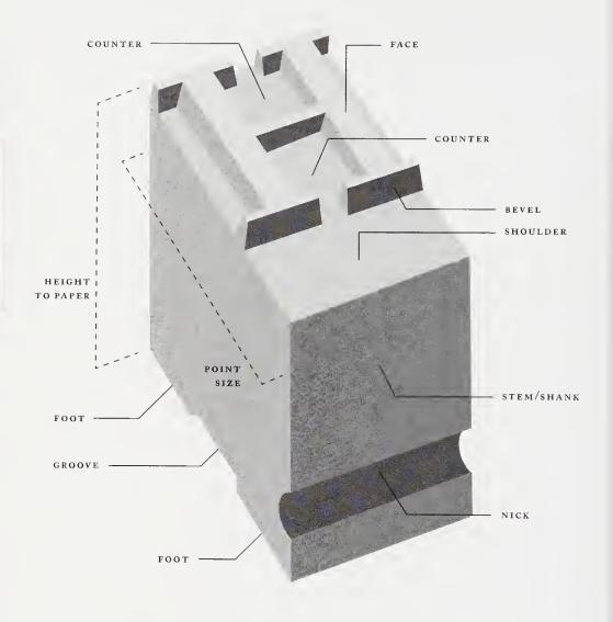
PARTS OF A CAST METAL SORT
