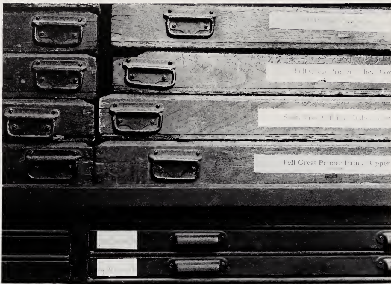
2. Oxford University Press's seventeenth-century Fell type is stored at Whittington in these large Barge cases and then transferred to standard cases for hand-setting. The drawers under the Fell cases contain the large collection of wood-engravings at the Whittington Press.
