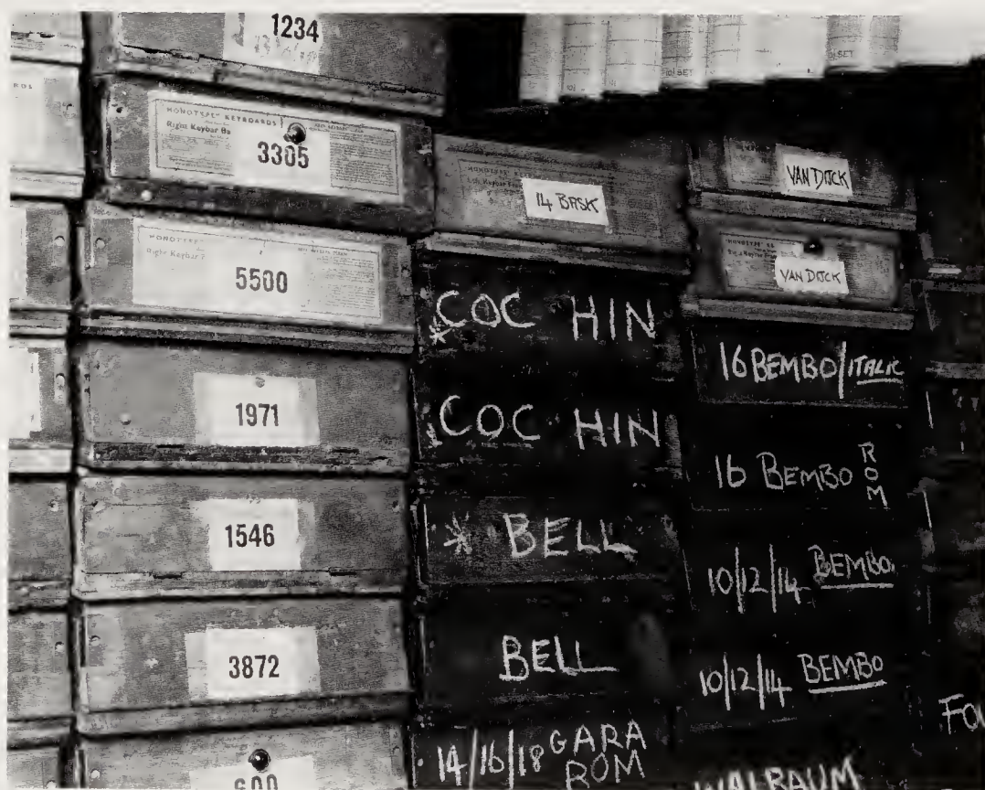
3. The keybars that control the operation of the Monotype keyboard are housed in these wooden boxes, with the name of the fount written on each box
