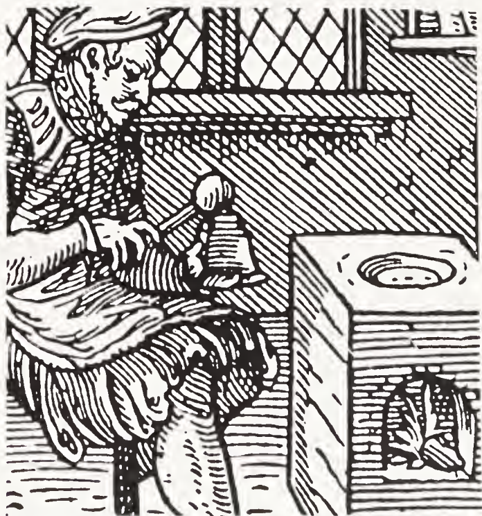
Typecaster pouring lead into mould: from an early engraving by Jost Amman (1568)
