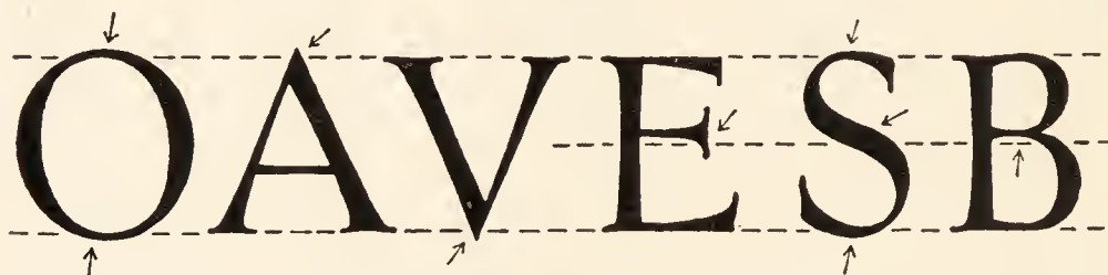
Fig. 18. Drawing of letters showing the head and base lines of serifs, and centre line. The arrows indicate where geometrical precision has been discarded for optical effect.
