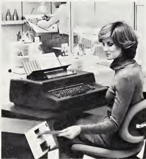
13-7. The MT/ST direct- impression typesetting system. Photo courtesy IBM
