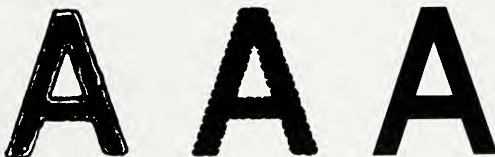
10-1. (from left) Results of relief, gravure, and offset lithography.
