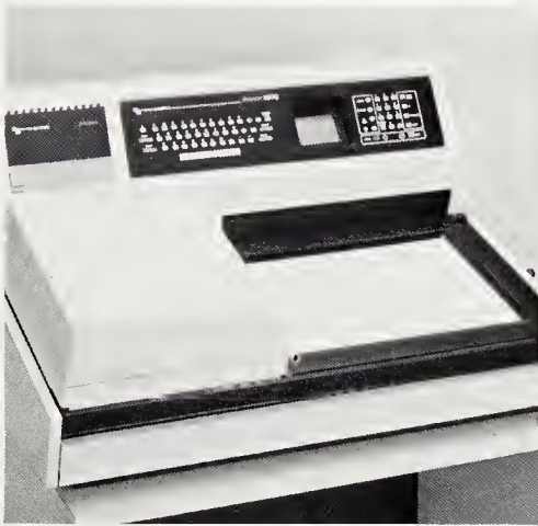
13-21. The Scanner 2000, an OCR device. Photo courtesy Compugraphic Corporation
