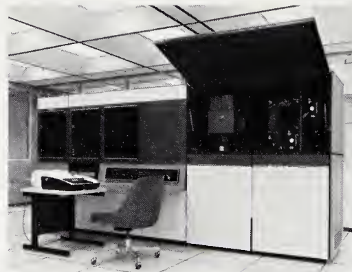
14-27. The COMp 808/3 Universal Pagesetter. Photo courtesy Information International
