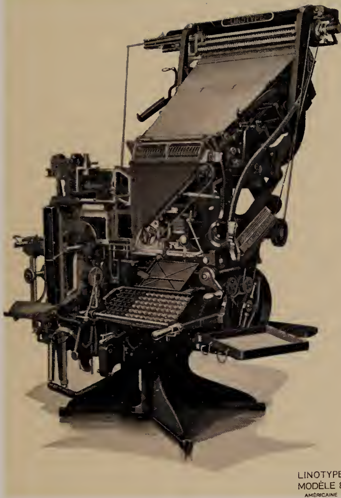
165 Linotype machine, Model 8, the United States.
