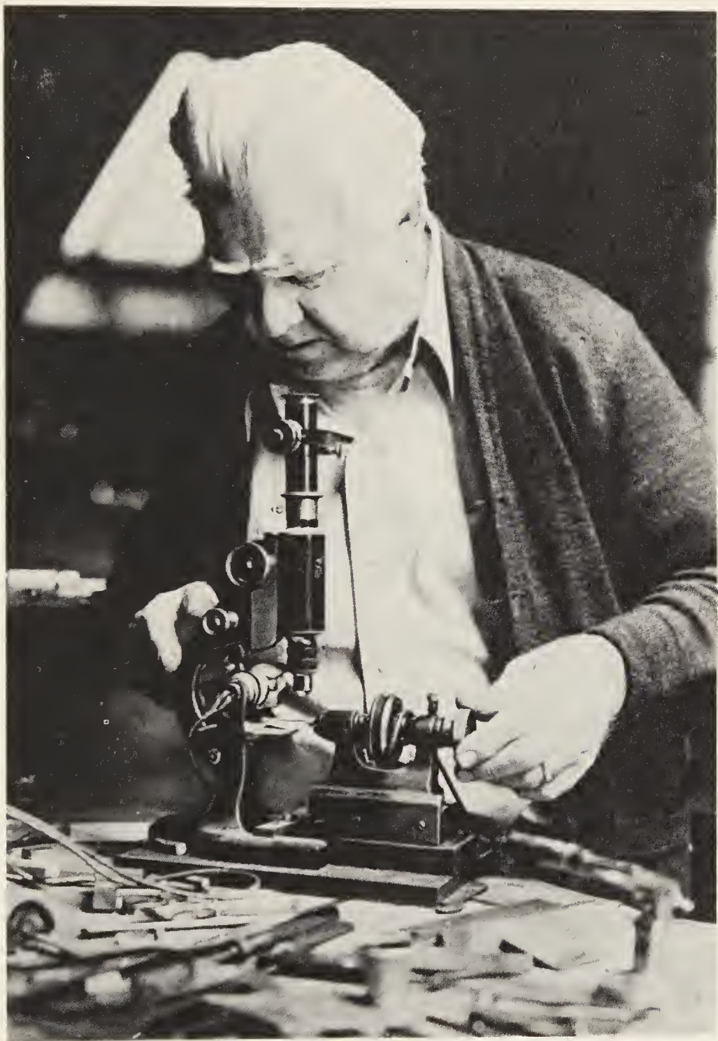
EXAMINING MATRIX CUTTER UNDER MICROSCOPE
