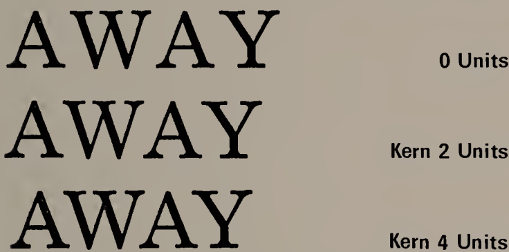
7-5. Reducing space between letters is called kerning, after the cutting off of metal on foundry type. Certain combinations of letters, when set with normal spacing, appear too open, and normal regularity is achieved by kerning.
