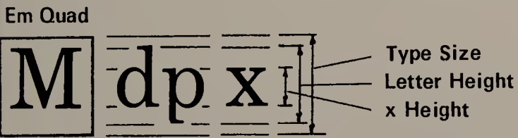
13-3. The relationship of letter size to type size is indicated by this diagram. The letter image may not always fill the type size. Many phototypesetting systems maintain base alignment of different font designs for mixing typefaces.
