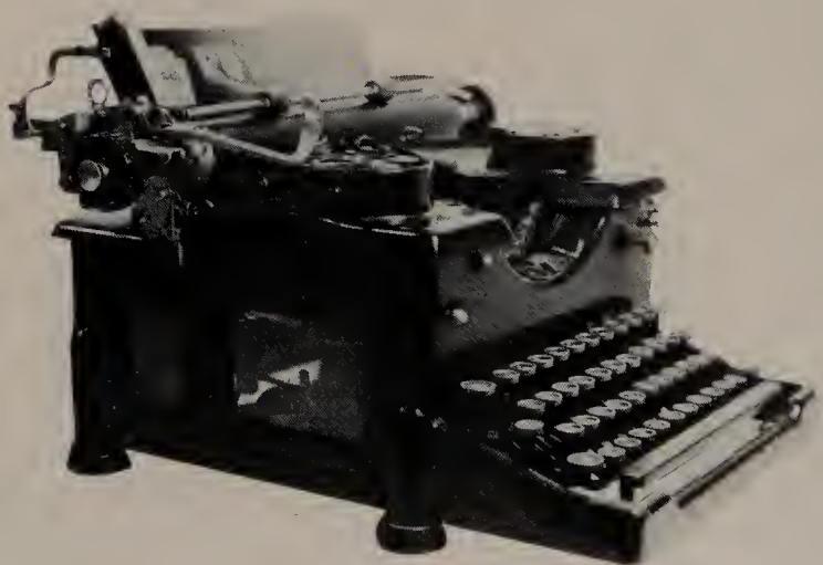
8-3. A typewriter ad from the turn of the century touted Visible Writing, Perfect Alignment, Automatic Action, and Ease of Operation. All the parts were exposed. A couple of decades later all the parts are enclosed, but viewing them and their action is made possible by the glass windows inset in the sides of the machine. It is quite a contrast to the black box of word processing.
