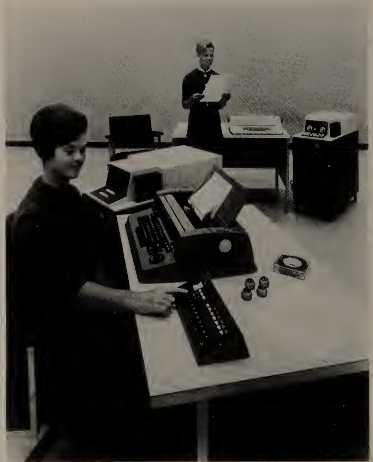
I-2. The term "word processing" was first introduced with IBM's Magnetic Tape Selectric Composer (MTSC). The system included one or more Magnetic Tape Selectric Typewriters (MTSTs), seen in the background, for recording the keystrokes of the manuscript. The tape is transferred to the record-reading unit at the left of the composer and played out at fourteen characters per second, about one-hundred and fifty words per minute, to produce typesetting composition. The typeset configuration or format is entered on the console in the immediate foreground.
