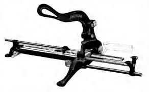
firmly in position by a strong spring. These teeth seat on their sides and do not touch at the bottom, which renders them self-centering and also compensates for wear, it being obvious that any wear in the teeth will merely permit them to mesh the deeper. The grooved bed makes it impossible for thin material to get under the gauge.
