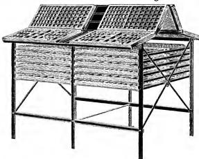
The Quadruple Stand has novel features. The cases on top project eight inches from the rack, giving the compositor plenty of knee room. The galleys between top cases are six inches wide, and divided into convenient spaces.
