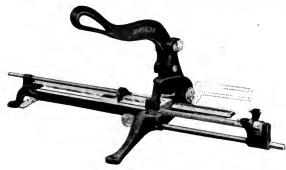
convenience in cutting odd or very short pieces; for instance, when in need of a few additional spaces for some odd body such as 14 or 20 point. they can be cut quickly and accurately with the aid of this device.
