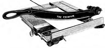
This is the popular, general, all-round machine, with a twelve-inch blade, meeting the requirements of a medium-sized cutter. A distinctive advantage is secured by a peculiar arrangement of the joint, by means of which a sheet of any length may be cut. By the simple adoption of a spring overhead, connected by a cord attached to the handle, the cutter is adapted to rapid work where a great number of small pieces of uniform size are to be cut.
