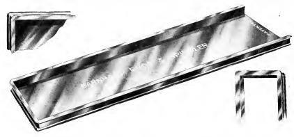
This all-brass galley has a rim of only one piece: a continuous strip of heavy flanged brass, formed to perfectly square corners inside, and secured to the bottom by more rivets than are used by any other manufacturer.
