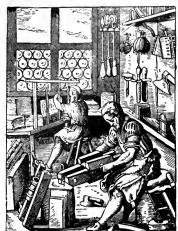
type is of one piece and is resting on a rude frame. All the boxes are represented as of the same size, but this is probably an error which is frequently made by designers of this day. The engravings of cases shown by Moxon have boxes of unequalsize. No doubt, they were so made from the beginning, for a day's experience would teach any
