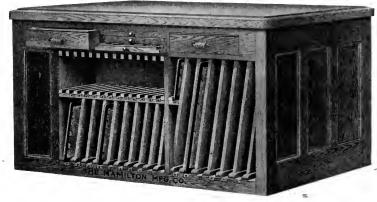
Chase Racks—One side of the Frame is taken up with Chase Rack equipment. There are 14 Racks 10½ inches in height by 12½ inches deep; 9 Racks 16 inches high by 19 inches deep; 6 Racks 20½ high by 18 inches deep. All of these Chase Rack compartments are lined with iron on the bottom turned at the edges to prevent damage to the wood work when heavy forms are pushed into the compartments.
