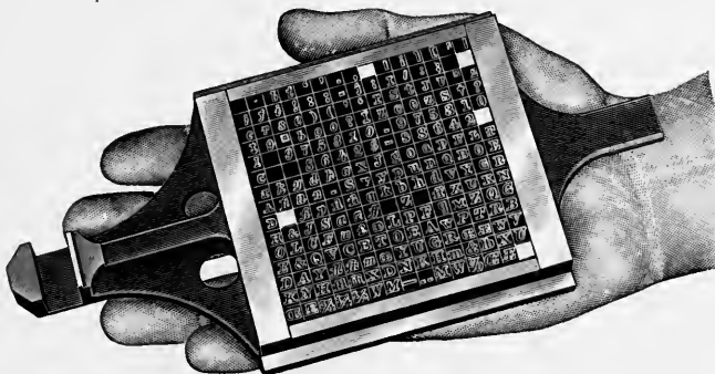
FIGURE 11—The Monotype Matrix Case, or "Magazine," holds 225 Matrices and weighs complete only thirty ounces
