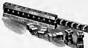
FIGURE 3—The comb and Matrices it carries. (Half Size)
