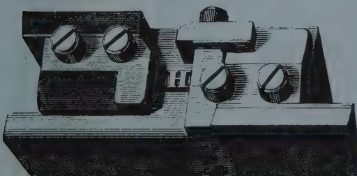
Type-mould without matrix, and with a type of the letter H in the mould.
