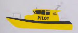
A pilot boat is a strong, fast boat that is usually painted a bright colour to make it easy to spot. It is used to transport pilots between land and the ship that needs piloting.
