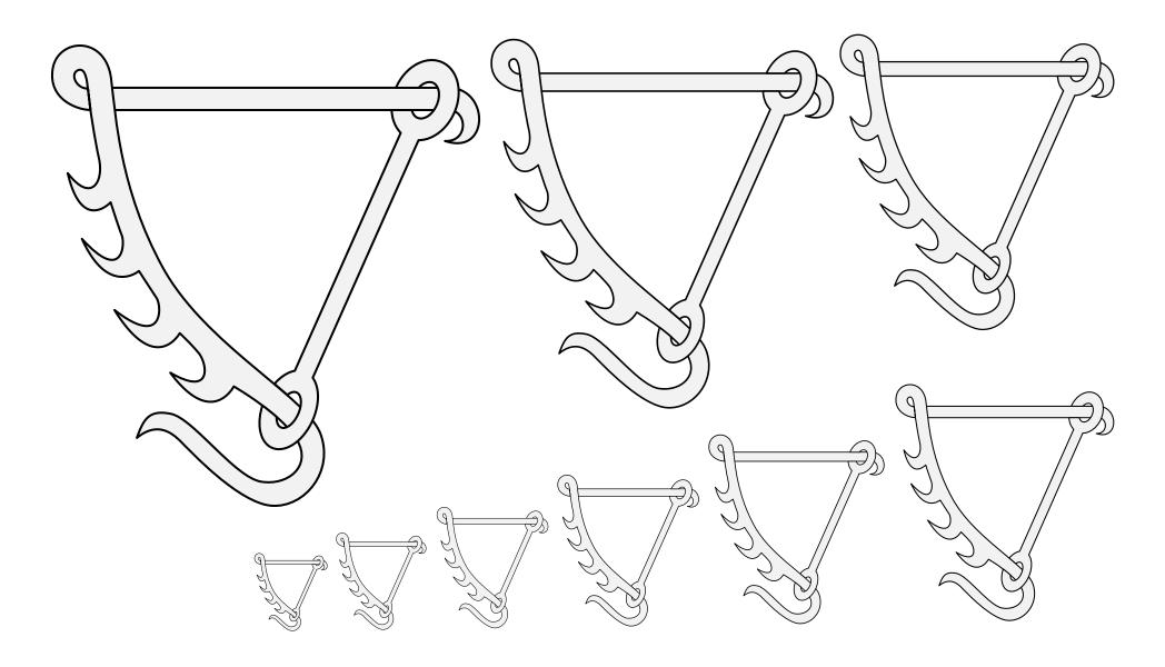
An adjustable hook for controlling the position of cooking pots above a fire.
