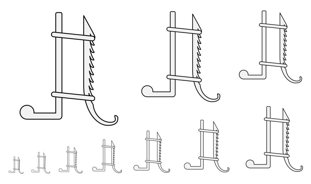
An adjustable hook for controlling the position of cooking pots above a fire.
