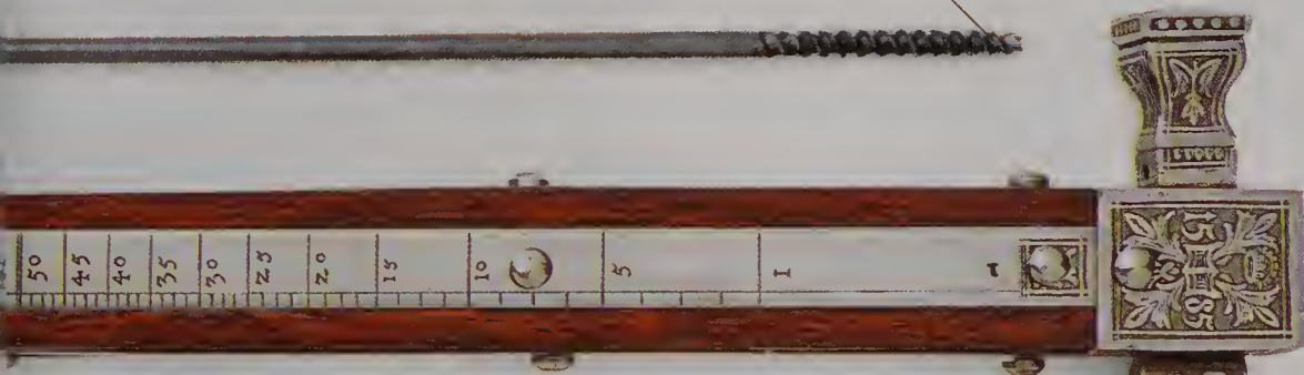
Screw for loosening powder encrusted in a cannon's vent
