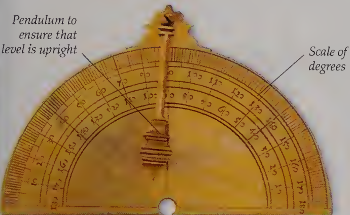
Gunner's protractor to measure angle of gun barrel
