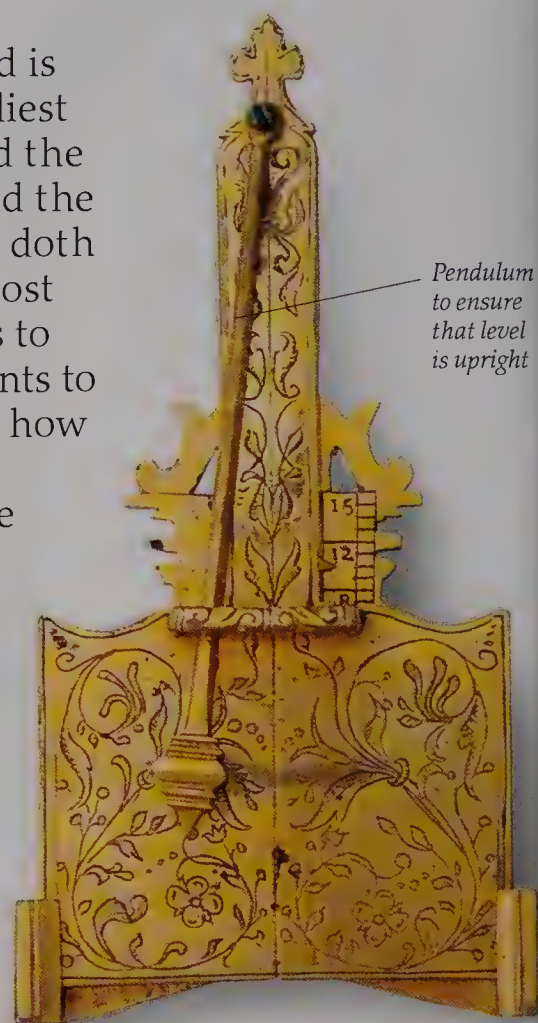
Gunner's quadrant, placed against underside of mortar barrel to measure its angle
