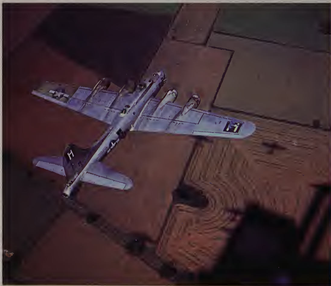
Note the camouflaged wing panel from an aircraft cannibalised for spare parts used to patch the flak-damaged port wing of this B-17, photographed near Snettisham in early 1944.
