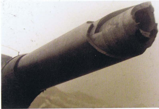
A close-up of the damage to the port forward 12-in gun barrel on the Orel . A hit from a large-caliber round shattered the end of the gun barrel, disabling this gun. (Naval Historical Center, NH66268)
