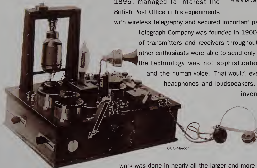
1914: Set used by Marconi between vessels at anchor 10km apart off Italy
