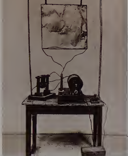
August 1895: Marconi achieves transmission over a distance of 1.75 miles using an earth and an elevated aerial at both the transmitter and the receiver
