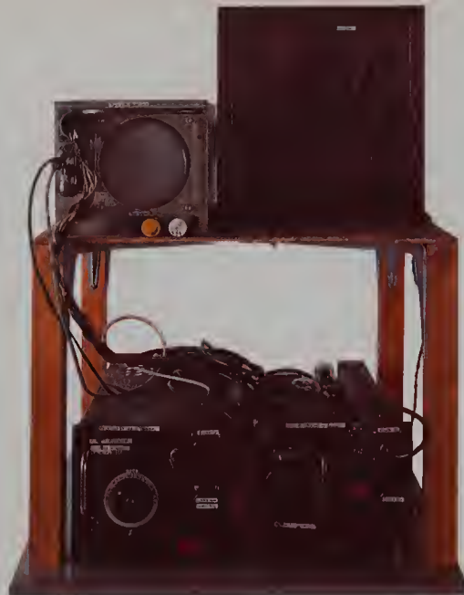
Home-made television set constructed from a Second World War airborne radar receiver, 1948
